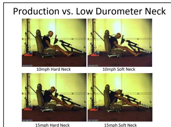
Figure 6. Comparison of the production and prototype flexible rollover neck at maximum head excursion.
