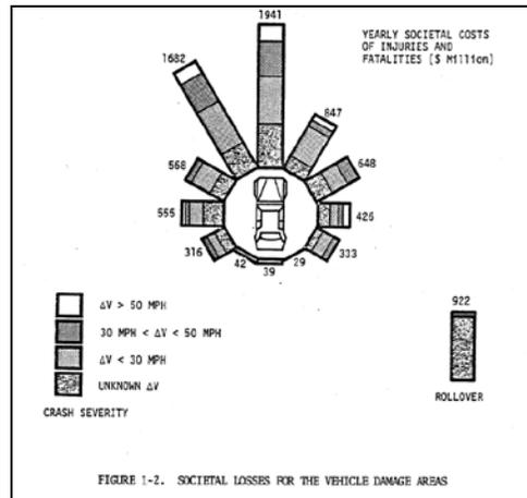
Figure 9. Societal losses as a function of deltaV and vehicle damage areas.
