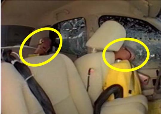
Figure 14. IIHS 2006 Crown Victoria side impact test (no airbags) at maximum head excursion.
